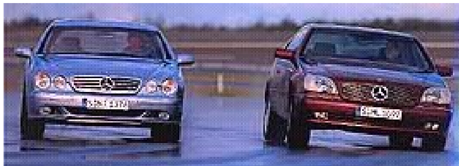
Figure 10: New Mercedes CL model using ABC versus older model without ABC [2]
